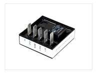
Smart and compact controller for 12V and 24V, that makes it possible to use the position light on the car, truck and trailer for indicators, and also use the indicators as position lights, also called US light.
