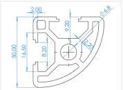
3030 profile that has been rounded on two of the sides, with 8mm tracks on the last two sides. The soft round edge makes it perfect for frames and enclosures.
