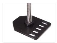
Collar that fits M8 lead screws, that is used for locking the screw in position, typically used in a lead screw plate. It is fastened with a pinol screw.
