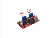
Compact regulator that can step down the voltage from 35V down to 1.5V, and limit the current from 2A and down.
