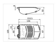
Smart box that can be put down in the front edge of a series 30 profile. Can be used for components, tools or similar.
