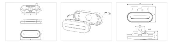
Nice marker lamp with LEDs in the middle and built-in reflex. The lamp is available in yellow, red and white and can be connected to both 12V and 24V. The powerful LEDs provide a clear marking on distance, and the reflector glass makes the car, truck or trailer visable - even when it's turned off.
