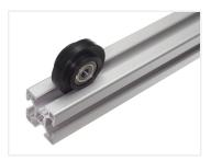
Wheel in hard plastic with a raised edge, that fits in to serie 30 and 40 tracks (8mm tracks). The wheel is used for guiding movable parts in the track of the aluminium profile. This could be a sliding door or similar. The wheel is made of durable nylon. The ball bearing ensures a smooth gliding motion, without wear.
