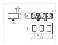
Smart roller-element module that is clicked on to a series 40 profile. Can be used for building gliding tracks or similar.
