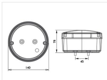
A bright 27W LED lamp built in to a standard Dasteri lamp with clear glass (140mm). Intended as extra reverse light, but can be used anywhere. The chrome-frame in the pictures is an optional accessory.
