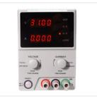
Powerful digitally adjustable laboratory power supply, 1 channel with max 30V and 5A. The voltage and current is easy to adjust with the two wheels, where a push on the wheel changes between which number is changed. The resolution of the voltage is 10mV, and the current is 1mA. The chosen setup is saved on restart.
