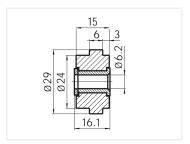
Wheel in hard plastic with a raised edge, that fits in to serie 20 tracks (6mm). The wheel is used for guiding movable parts in the track of the aluminium profile. This could be a sliding door or similar. The wheel is made of durable nylon. The bushing that is hammered in to the wheel is zinc plasted steel.
