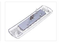
LED emitters 24V that replace the original circuits in the top lights on the new MAN trucks. The original emitters are taken apart by removing two metal clips, where after the board is taken out and the new put in.
