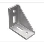
Extra large angle bracket, that gives extra stiffness and strength in the connection, compared to standard. There is space for 4 pcs M6 bolts in the bracket. You should use 14 or 16mm bolts together with a washer.
