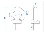
Stong liftingeye / ring that can be used for hanging or lifting parts. Can be used in connection with system profiles. Available with M8 thread.
