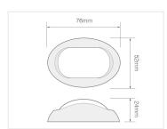
Great looking LED marine boat lamps in tear shape, with white or chrome house. With red, green and white glass and LED light, that will never require a bulb replacement. The manufacturer offers 5 year waranty on the lamp, and the construction ensures that the lamp will endure many seasons. Easily mounted on the boat, without any visible screws or bolts.
