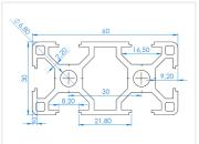
Strong alu-profile with basis dimensions 30x60mm, with two tracks on one side, and one on the other. The double width compared to the standard profile makes it extra useful for primary posts in constructions, or when you need two parallel tracks.
