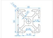
Standard profile in series 30, with basis dimensions 30x30mm and 8mm slot / track width. These profiles have a medium strength, and are a great choice for many types of constructions, such as CNC machines and automation tasks. The profile can also be used for CNC mills and automation tasks. The profile can also be used for shields, enclosures and similar.
