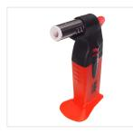
Large professional handheld gasburner for shrink tubing, solder sleeves, soldering and similar tasks. The gasburner has piezo ignition and wheel for adjusting the flame size. It is possible to lock it on on after igntion, where after it can run about 1 hour on a full tank.
