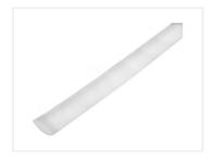
Shrink tubing in transparent plastic, that can be used for clear joints, eg. on splashproof LED strips. The tube shrinks 2:1 in diameter when heated with a lighter, gasburner or hot-air gun.
