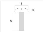
Standard M6 bolt in various lengths, with round unbraco head. Used for nuts with M6 thread.
