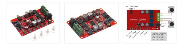
Amplifier module with built-in Bluetooth and analogue input (3.5mm plug). The module can play music and other sound wireless over Bluetooth 4.0 from smartphone, tablet and PC. The amplifier has 2 outputs of 50W outputs.
