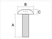
Strong M8 bolt that fits in to parts with M8 thread, and in the ends of serie 40 with cut threads. Available in 25mm and 30mm lenghts.
