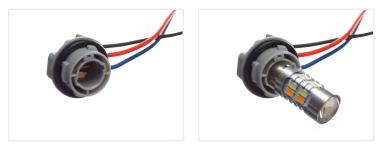
Base for BAY15D bulbs, with wires for connection. The gasket on the lamp secures a waterproof joint in a 26mm hole. There is 120mm cables in the end.
