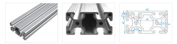
Extra strong double-width series 40 profile, typically called 4080, that eg. can be used as a basis frame in a larger constructon. There are 2 tracks on both sides, and 2 in the ends, with a total of 6 tracks, 8mm. There are also 6 holes that you can cut a thread in.
