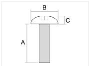
Standard M5 bolt in various lengths, with round unbraco head. Used for nuts with M5 thread.
