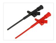
Smart probe for clipping on wires or components on a circuit. The clamp opens when you push in the end, where after you can put the wire in and then release. The wire will then sit securely clamped.
