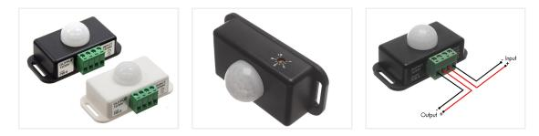
Compact PIR motion sensor with screwterminals on the input and output. The sensor can be used for both 12V and 24V. When the sensor is activated, it will turn off after the set up delay, that can be from 1 to 10 minutes.
