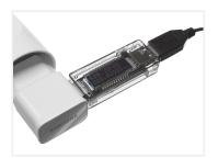
USB charging-tester, that measures and displays charged capacity, charging voltage and current in the large display.
