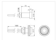
Small powerful 24V RGB LEDs, mounted chrome or black metal frame with long thread. Used for interior decoration, plushing etc. in trucks.
