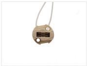
G9 socket in ceramic that fits standard G9 bulbs, both halogen and LED. There are premounted wires on the bottom.. Easily mounted with 2 screws in the base of the socket. You only need to drill two holes for the wires.
