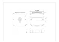
ECE-approved trailer lamp with a tail, a brake, and an indicator light in a classic look. The lamp has 4 red high power LEDs and 4 amber high power LEDs for respectively running lights and indicator lights. The lamp is also available with a built-in license-plate light, so you avoid mounting extra lamps for the license plate.
