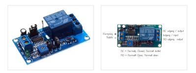
A smart relay with an adjustable on or off function. The delay can be adjusted from 0.1 second to 1 hour. The relay has one input and an output that is normally connected (NC) and another output that is normally open (NO).
