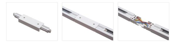
A joint for two tracks with inside screw-terminals for connecting the profiles to 230V. The two ends are pre-connected with cables and so this part can also be used as a simple joint.
