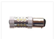
A very bright BAY15D bulb with 16 powerful 5W LEDs from CREE. Special optics create a wide light beam. The bulb has a built-in high and low beam function, where the low beam brightness is equivalent to 10W and the high beam is equivalent to 40W. An original BAY15D is 5W and 21W, so this bulb has a quite strong beam. The real consumption of the bulb is 8~10W.
