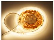
Powerful 24V LED stripes with a warm white light and with LEDs that have a high color reproduction (CRI). The stripes are made of small circuits in series, so you can cut the stripe, where marked. You can see the lengths of the circuits in the LED stripe data below.
