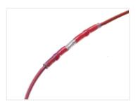
Solder-sleeves gives you secure and waterproof joints between wires. You can heat it until the solder melts and the crimp closes around the wires. The colored rings are glue that melts, and secures a waterproof joint around the wires.
