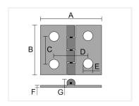
Plastic and aluminum hinges, that can be used for doors and lids. The hinge is fastened with M6 bolts.
