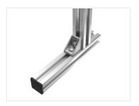
A bracket in aluminium for joining two series 20 profiles in 90 degrees. There are knobs under the brackets to keep them in the slot while tightened. The knobs can also easily be ground down, if you need to mount the brackets transversal.
