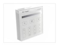
A light dimmer for 12V and 24V such as LED strips, that is easily controlled wireless with a remote, touchpanel or a wifi bridge so it can be controlled with your smartphone using an app. The controller has 2 output where each can draw up to 6A, total A is however max 12A. The receiving distance is maximum 30 meter.
