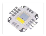
A very powerful high power LED with 4 color channels (RGBW / RGB + White), each shall be provided with 300mA-350mA. In each color channel, there are three strong LEDs in series. With a scattering angle of 140 degrees, it gives a very bright light. It has a life of 50,000 hours.
