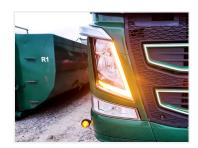
Complete set LED emitters for retrofitting your Volvo FH with amber or warm white DRL, or simply for replacing your emitters if one of the original break. These fit Volvo FH from 2012 and forward. There is in total 20 or 10 LEDs per set with a total output of 2000 Lumen. The output is equivalent with the original.
