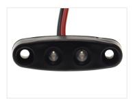
Matronics Flexbox 2 is an extra small LED lamp with 2 powerful LEDs. The lamp is potted, so it is completely waterproof. It can be mounted both indoors and outdoors, on both cars and trucks. The lamp has a built-in voltage regulator, so it can be connected to both 10V and 30V.
