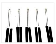
3 mm diodes with integrated resistance, which means that you can connect 12V directly to the diode without a dropping resistor. 60 degree dispersion angle. It is suitable to build it in contacts etc., where the bulbs cannot be swapped out with a diode bulb.
