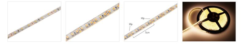
The splashproof LED Tape SMD can be shortened or extended further, so it fits for your project. The stripe is 8/10 mm wide and is built up in small modules of 5 cm or 10 cm, where there are 3-6 heavy SMD diodes in a circuit ready for 12Vdc. There are clear markers where the stripe can be cut, as well as solderislands, where you can solder wire on or extend with more SMD-tape. On the back is a 3 m powerful tape, which makes that LED SMD tape to stay attached to his seat without screws.
