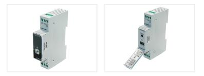
In the process of switching to LED, certain dampers can have problems with the lower power consumption. Niko's universal dimmer takes care of this and makes it possible to swap the existing tablet dimmer or the impulse switch. The low requirements for a minimum consumption and the special engineering enables the control of dimmable 230V LED bulbs and of iron core transformers for 12V LED bulbs.
