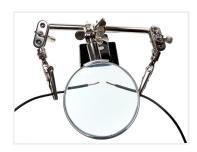
Ideal for all kinds of fine electronics work, where both of your hands are busy, for example with soldering. 2 arms, which can be moved in all directions, with alligator clips.
