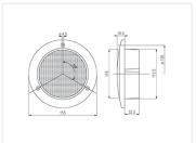
24V rear light with turn signals brake lights & backlight. A ring of red diodes for rear and brake lights and an orange diodes in the middle for the flashers.
