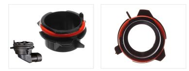
Is your BMW E39 equipped with Sockets as shown in the buttom of picture 1, and uses H7 bulbs, then you can buy this adapter set which makes the fitting easier of our H7 Xenon kits.
