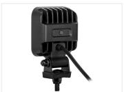
E-approved LED lamp with 12 powerful Osram LEDs. Aluminum housing with durable powder coating and stainless steel brackets. The light color is 5700K, and the 90-degree optics provide good and broad light distribution.
