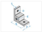
Corner bracket in solid aluminum, with M6 sidehole, which can be used for feet, wheels, or to attach a plate. The bracket is typically mounted at the bottom of a frame, where it is fastened with two M6 bolts.
